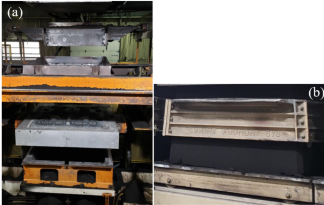
Figure 1: Molding lines at Erie Bronze and Aluminum Company: (a) automatic, and (b) manual. Published with permission.
