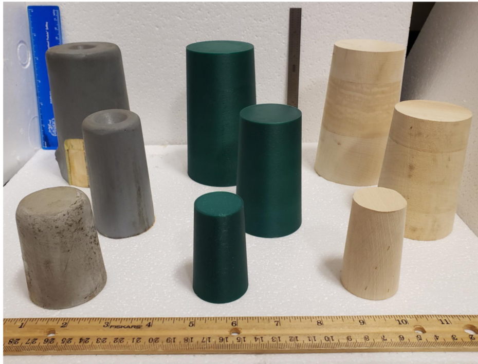
Figure 7: Old wooden risers and new wooden risers next to their printed plastic counterparts at each of the three scales.
