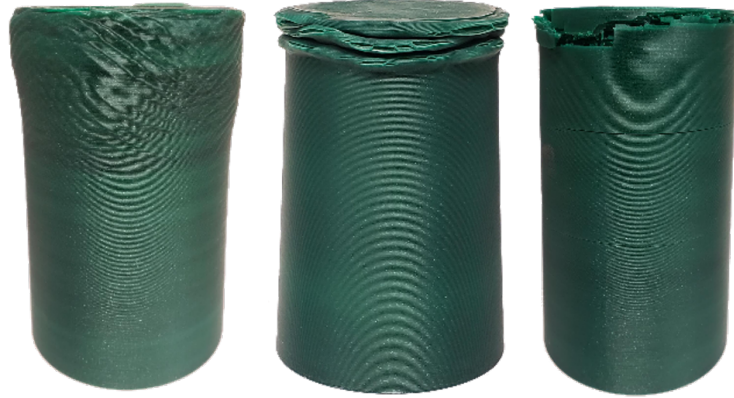
Figure 15: Plastic failure modes: compression (left); layer collapse (middle); brittle crack (right).
