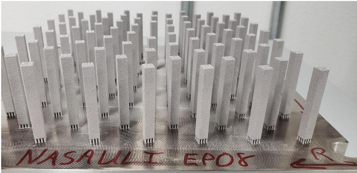
Figure 3: Image of EP08 samples on build plate
