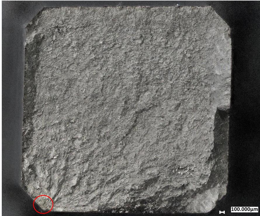
*Figure 15: Sample F49 - Initiation site on the lower left side chamfer*
