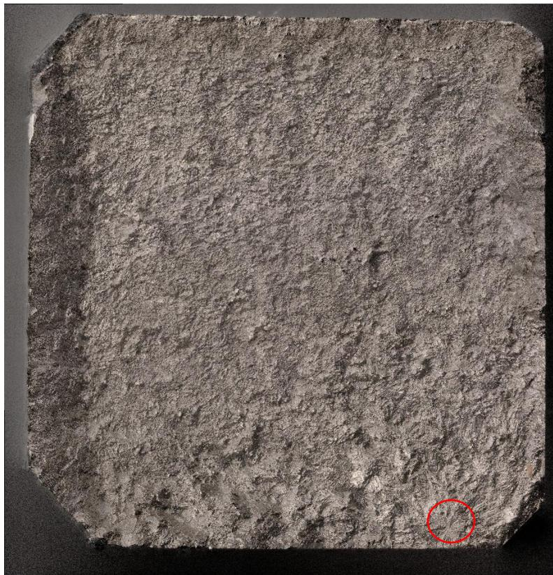
*Figure 16: Sample F77 - Initiation site at defect on the lower right side*
