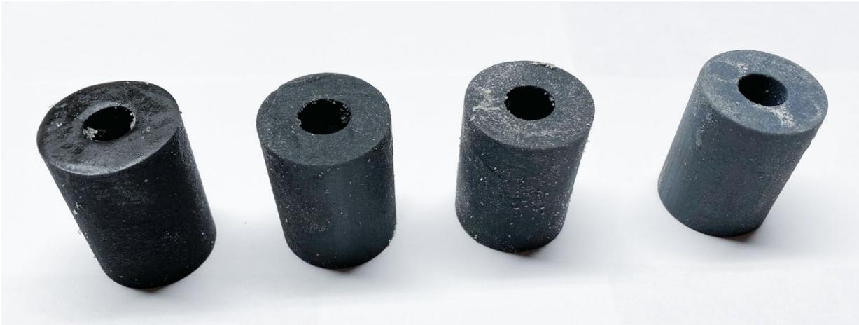
**Figure 1:** Polymer Suspension components. From left to right, 25% liquid, 40A, 60A, and 95A
