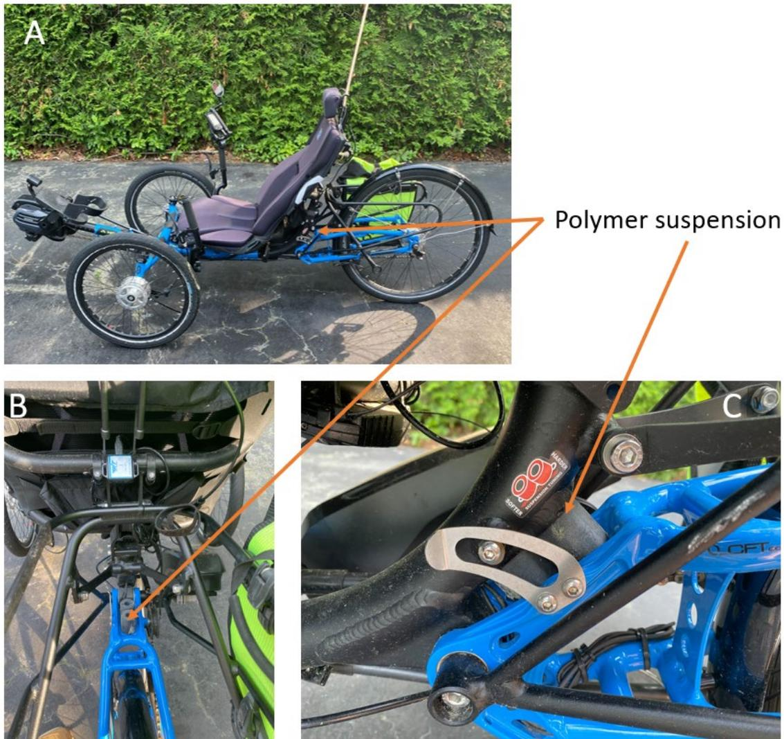
**Figure 2:** The ICE Trike(A) with the polymer suspension system. The rear suspension is blue in parts B and C. The polymer components are attached to the suspension and compress on the front frame.
