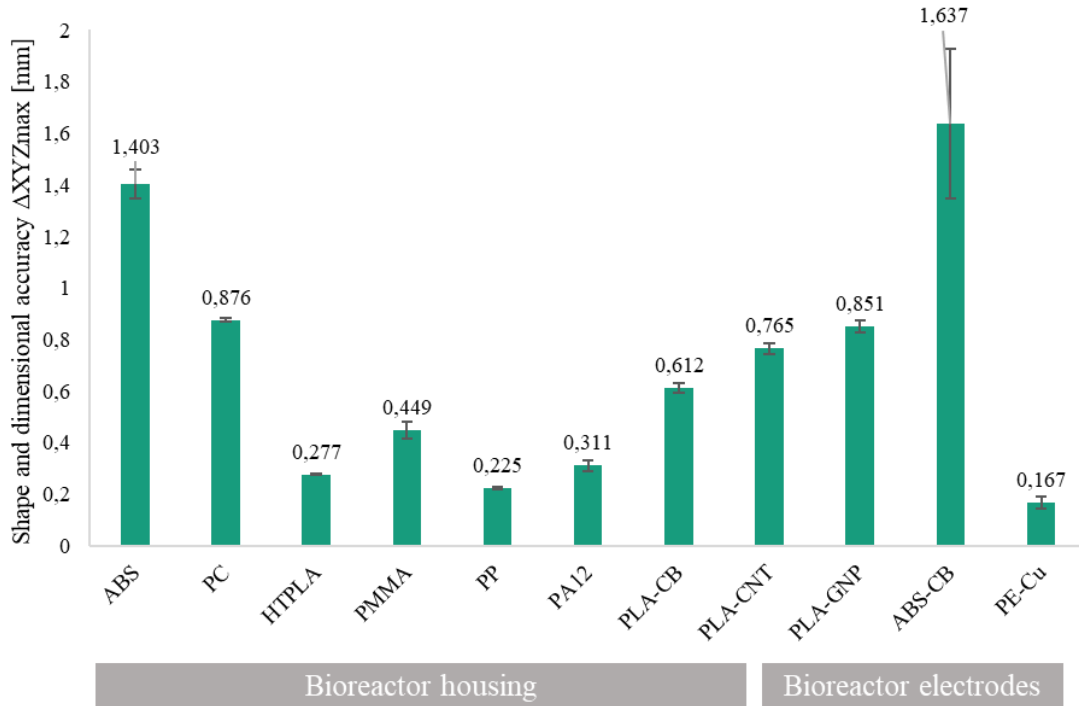
Figure 11 Results of high-temperature resistance of pre-selected materials for bioreactor housing and electrodes
