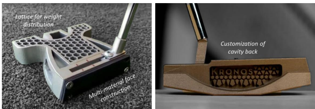
Figure 3. Examples of Opportunistic DfAM in AM Putters (Adapted from [48] and [49])
