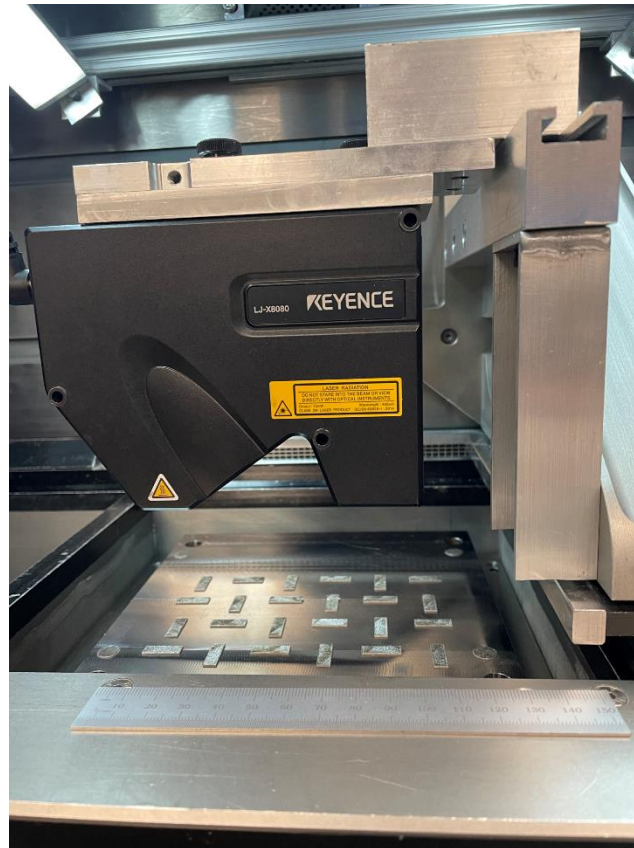
Figure 4: Keyence LJ-X8080 setup in EOS M280 capturing the part surfaces of experiment 1
