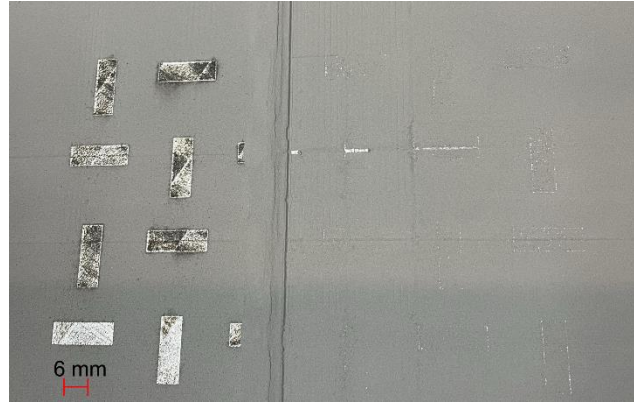
Figure 5: Location of build failure region in experiment 1
