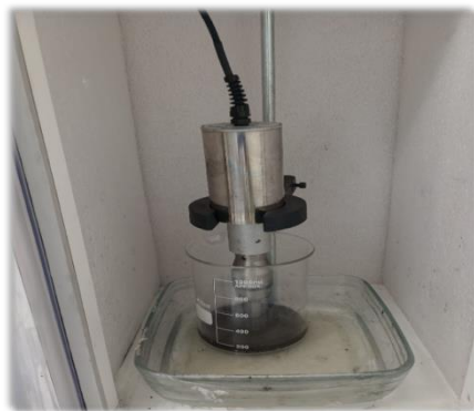
Figure 2. Probe sonication mixing
