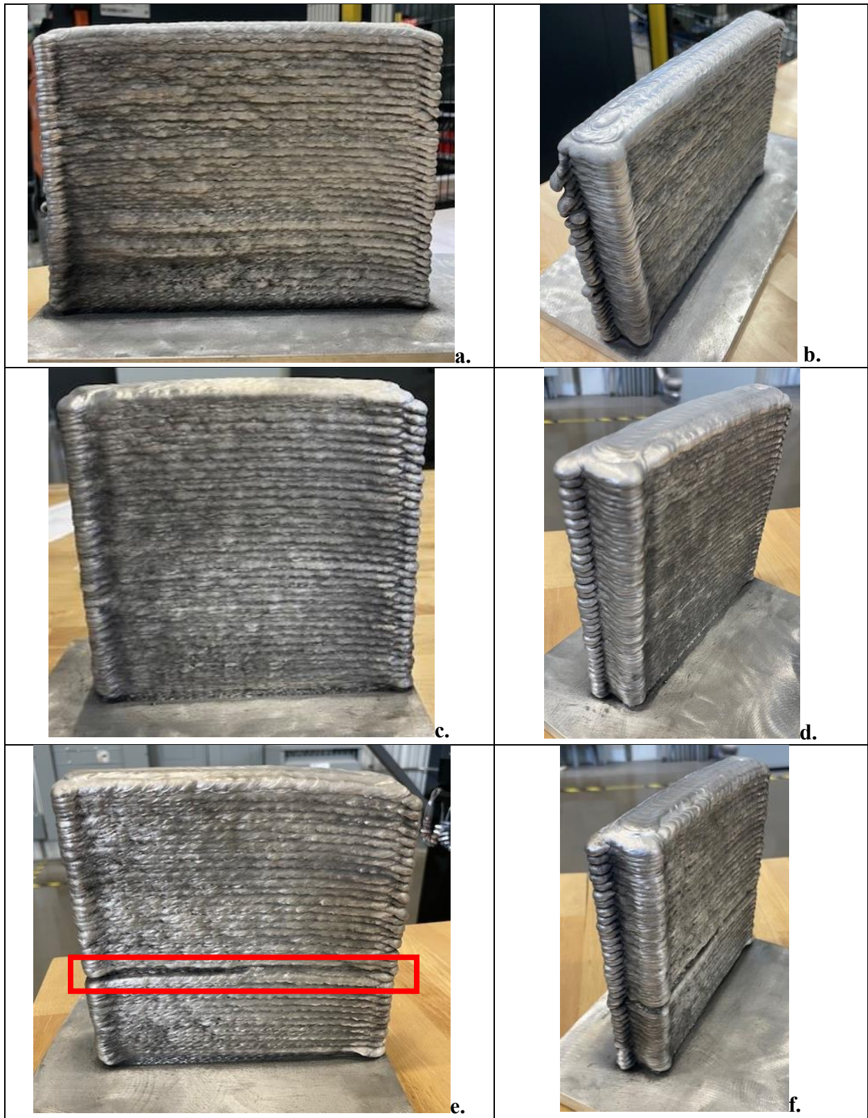
Figure 11 – Front and Isotropic Views of Three Spiral Path Test Blocks
