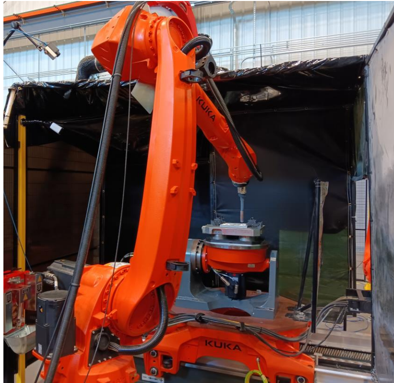
Figure 1: Hybrid cell: 6 DoF robot and 3 DoF positioner
