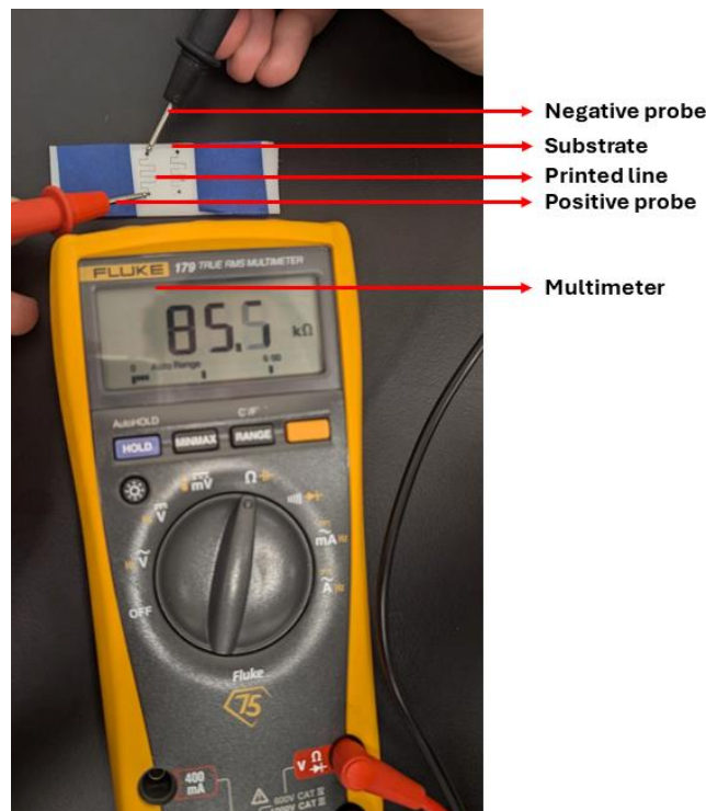
Figure 3: Measuring the resistance of the circuit with a 2-point probe.
