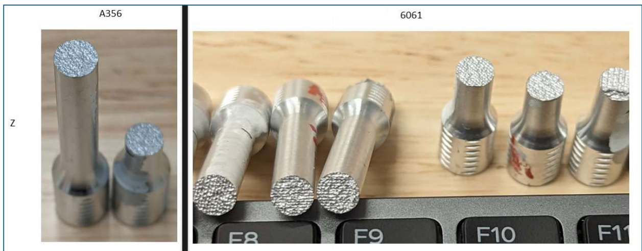
Figure 6: Left, Al A356 fracture behavior for the Z-build direction. The fracture occurs on the layer boundary. Right, Al 6061 fracture behavior for the Z-build direction. The behavior is very similar to the A356.
