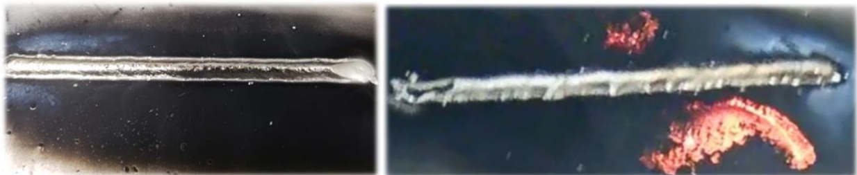
Figure 4: (Left) MIG Titanium Deposits with Soot By-Product, (Right) Titanium Soot Deflagration/Combustion
