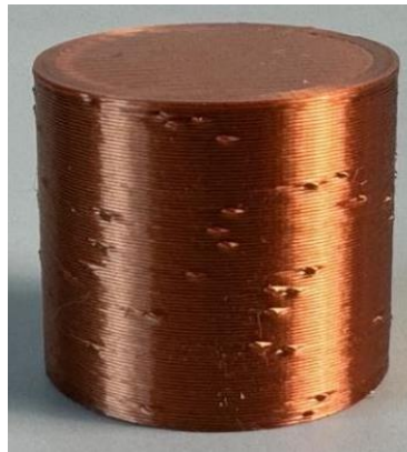
Figure 15: FDM printed cylinder with random seams showing like "zits" around the exterior surface.
