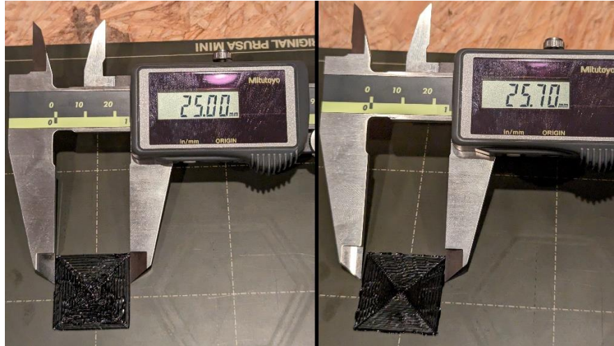
Figure 6: A 25mm square printed outside in (left) and inside out (right). Notice that the outside in square (left) perfectly matches the dimensions while the inside out version (right) is oversized because of the material being pushed outward during printing.
