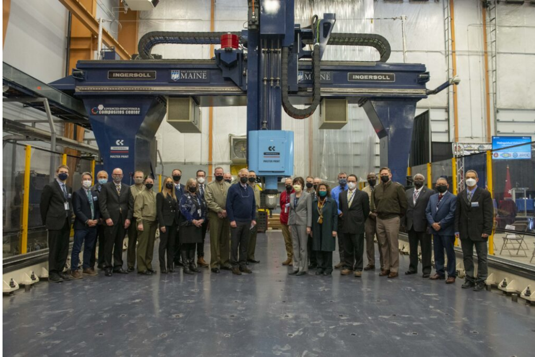
Figure 1: World's largest 3D printer at UMaine's Advanced Structures and Composites Center with a build volume of 100 \times 22 \times 10 feet, reproduced from [5].
