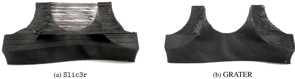
Figure 5: A 2.7 inch gyroid section sliced using Slic3r with retraction off versus one processed with GRATER on a desktop filament MEX AM system. Note the excessive amount of stringing between the two regions as a result of excessive travel moves.
