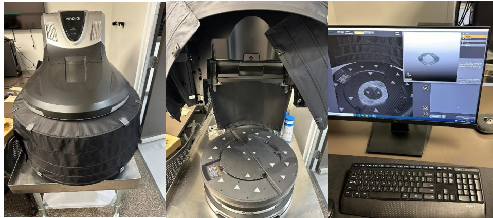
Figure 4: Keyence® VL-770 3D scanner
