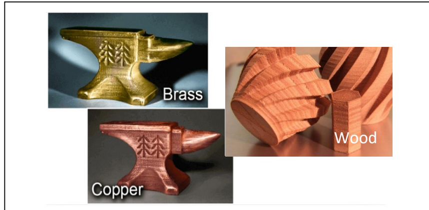
Figure 1: Material Extrusion Samples Produced with Polymer Composite Materials
