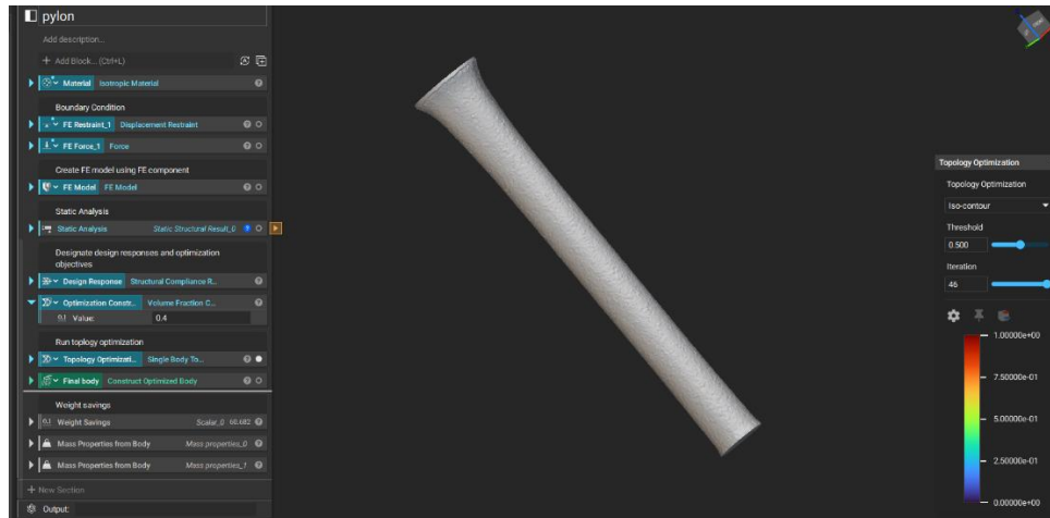
Figure 11. Topology Optimized rough part
