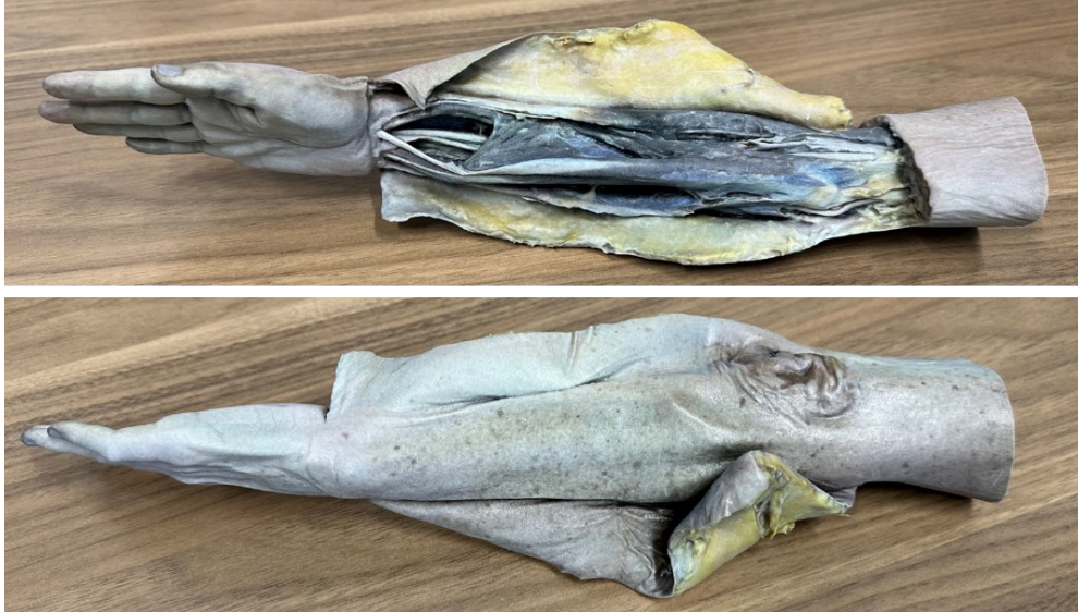
Figure 7. Final Manufactured Cadaveric Arm via Stratasys J55 PolyJet
