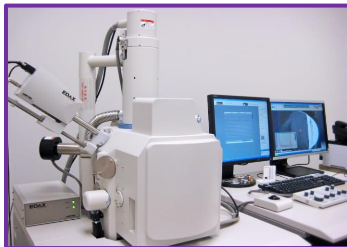
Figure 6: Test setup on SEM
