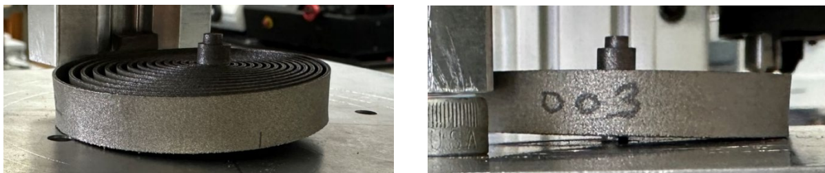
Figure 10: Springs under test experiencing cross-section twist.
