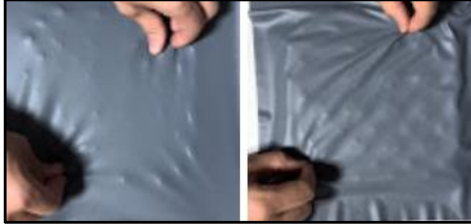
Figure 8. The lattice can be covered with a thin rubber skin to give a soft and conformal interpolating surface.
