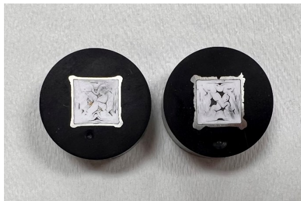
Figure 3-Cut and mounted samples deposited with (left) and without (right) Caswell
