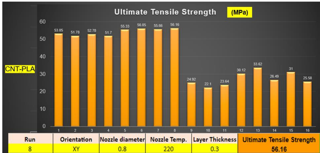
Figure 6. UTS of CNT-PLA with varying printing parameters.
