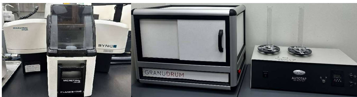
Figure 1. From left to right: Microtrac MRB, GranuDrum, and Autotap tapped density tester.
