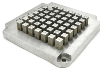
Figure 3. SS316L cubes for density measurement on the Seurat prototype machine build plate.
