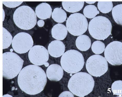
Figure 3. As-polished ATI Ti-6Al-4V powder optical image.
