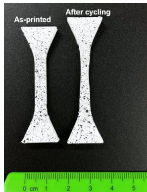
Figure 13. Comparison of an as-printed DIC specimen with one that was subjected to the shape memory cycle.
