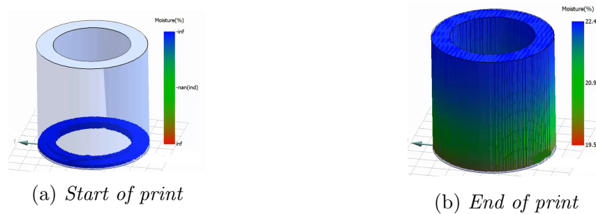
Figure 7: Moisture simulation at different stages of clay 3D printing
