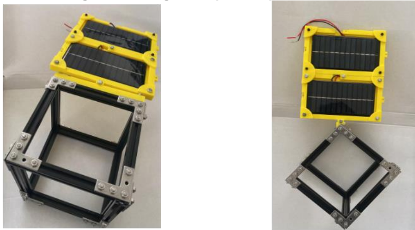
b. Solar Panels mounted 45 degree with respect to the member
