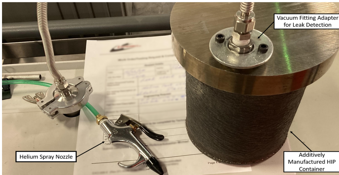
Fig. 4 Vacuum testing setup with DED manufactured cylinder with connected baseplate on top.
