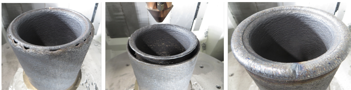
Fig. 5 Fabrication results: (left) after completing inner half arch; (middle) after completing both arches but with gaps remaining; (right) after final bead for complete seal.
