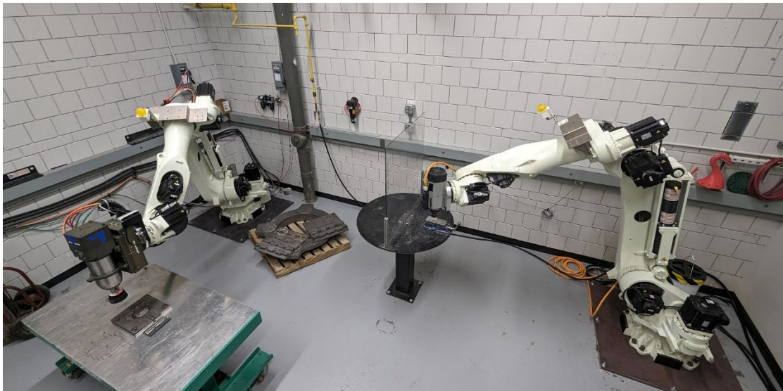
Figure 2. The robotic manufacturing cell at Iowa State University with Kawasaki CX165L grinding robot (left) and CX110L hybrid manufacturing robot (right).
