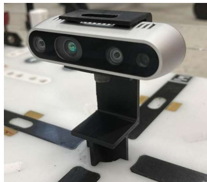
Figure 5: Side profile camera mount.
