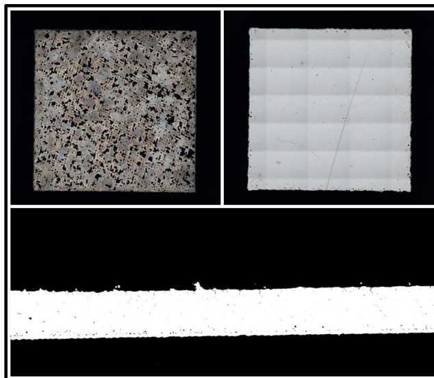
Figure 2: Defect pattern in the final part; low density (top left) vs. high density parts (top right); surface roughness (bottom)
