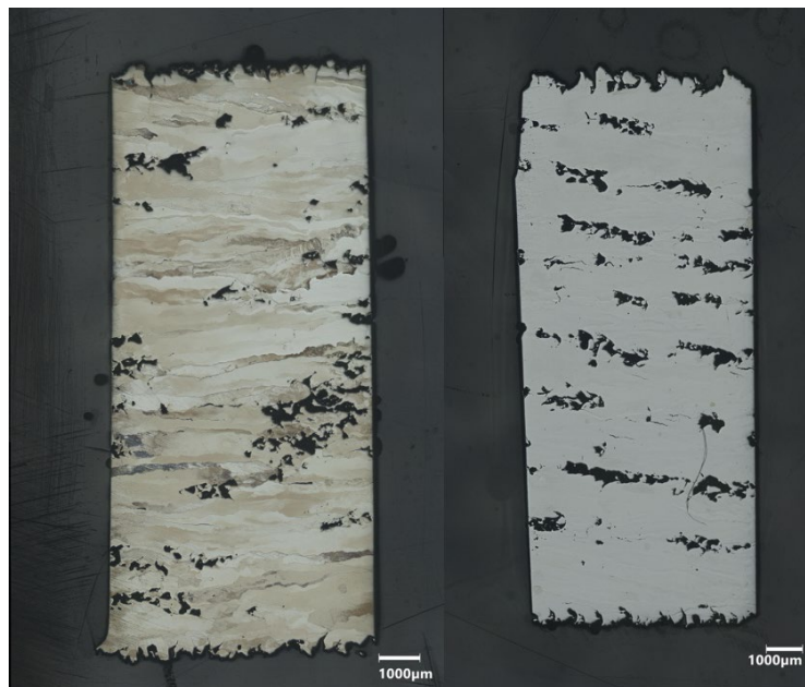
Figure 5 – Stitched micrographs of samples 5 and 6 on HIP 3, where lack of fusion is still present.
