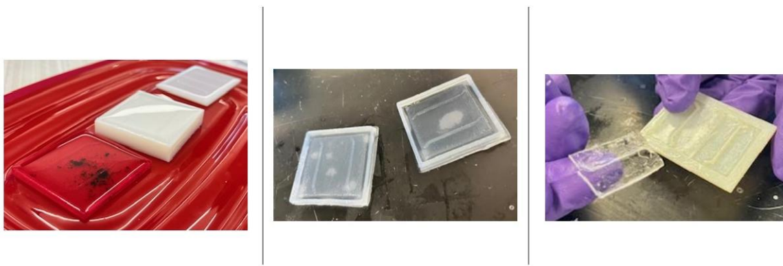
Figure 7. Molding Process chip. Left: Curing Resin parts in the mold. Middle Semi-cured resin molds: High-resolution print of the mold using resin jetting. Right: Cured PDMS ripped from mirrored mold.
