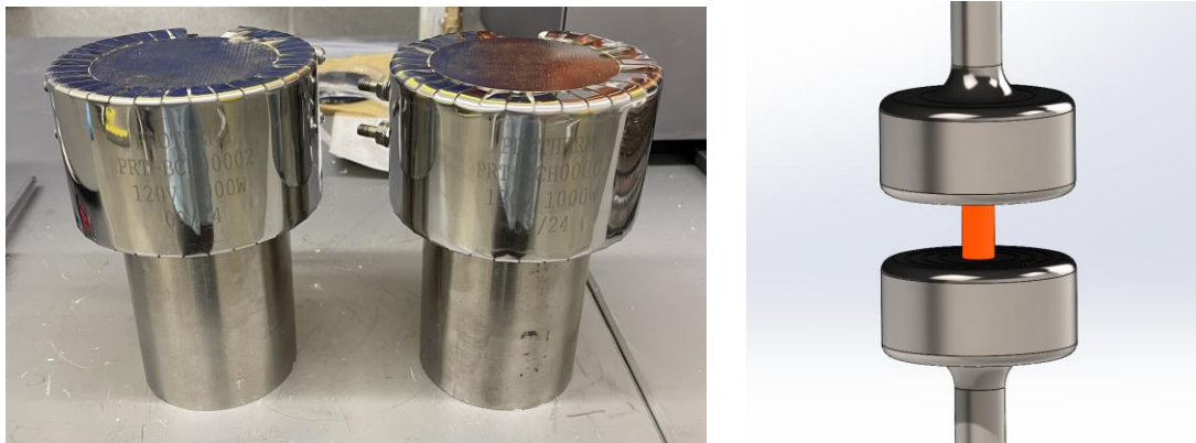
Figure 11. Platen before machining (left) and designed Platen and compression sample (right)
