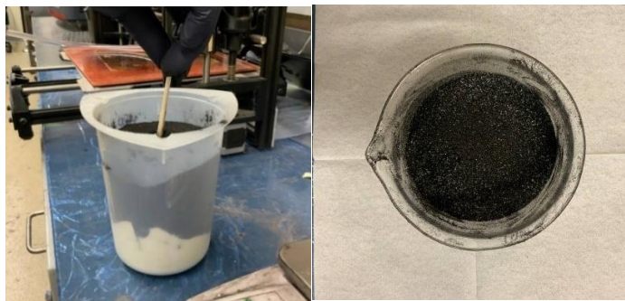
Figure 2 Hand Mixing of powdered plasticizer with PA 4,6 powder
