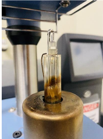
Figure 7: Mounted CTE sample on the TA Instruments TMA Q400
