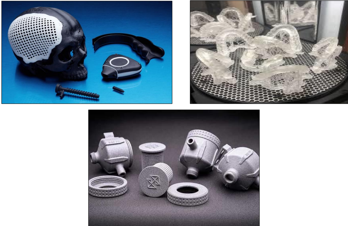
Figure 1: Stereolithography 3D printed materials for bio-medical devices, soft-robotics and electronic components
