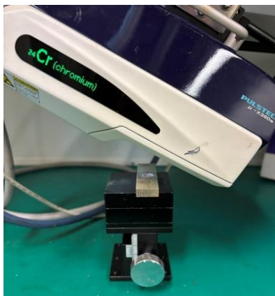
Figure 7. Pulstec micro-X360 x-ray diffraction system to measure residual stress in hybrid AM.
