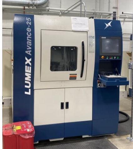
Figure 3. Matsuura Lumex Avance-25 laser powder bed fusion system.
