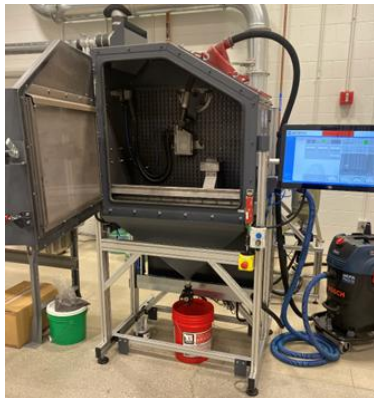
Fig. 5. Shot peening system used for interlayer treatment.
