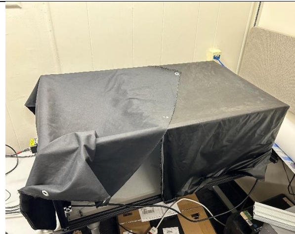
Figure 7 Hybrid neuromorphic imager-in-the-loop setup for generating simulated data for neuromorphic imagers. Outer Musou black felt covering is used to reduce stray light entering the system.
