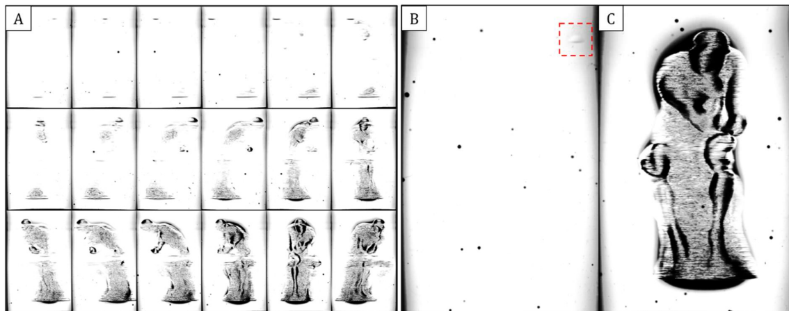
Figure 7: Polymerization progression during printing. (A) Timelapse of print, in increments of approximately 3 seconds from curing onset, (B) first visible sign of curing, (C) finished print suspended within the photopolymer in the print vial. While the polymerization progression of only one print is shown, the head of The Thinker was the first region to begin curing in all prints.
