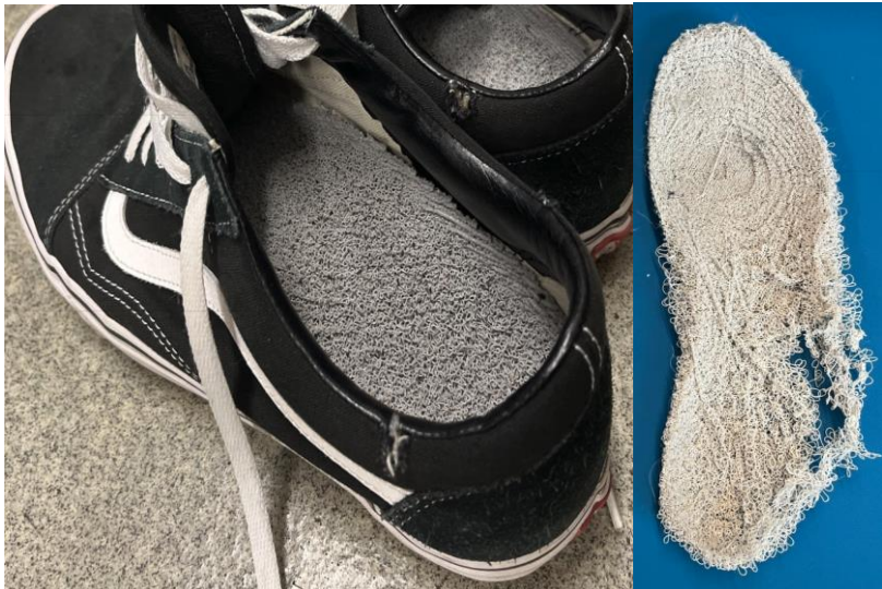
Figure 8. (Left) Shoes with VTP TPU insoles. (Right) Insole after 50,000 steps
