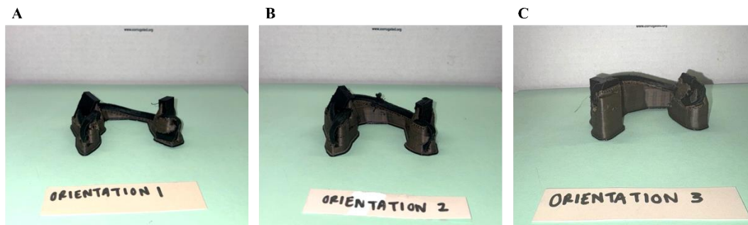
Figure 9: Printed specimens of the following orientations: A) Auto, B) XY, and C) XY-180.
