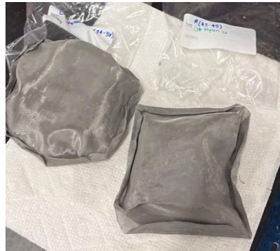
Figure 10: Example of specimens wrapped in stainless steel mesh bags to be placed in the SCA.
